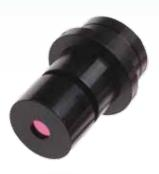
The DinoEye AM7023 is equipped with a 5 megapixel sensor for crystal clear images. The AM7023 is the ideal solution for displaying microscopic images on large screens. The DinoCapture software is bundled with the product. It fits into 23 mm microscope oculars. Also available to fit a 30 mm or 30,5 mm microscope ocular (Dino-Lite AM7023B).
