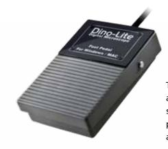
The SW-F1 is a foot pedal which allows you to take a picture with a simple step from your foot. Simply plug in the device into your USB port and it is ready to use.
